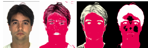
Figure 3: From left to right: original face, K-means classifier output for H channel, K-means classifier output for S channel and K-means classifier output for V channel.
