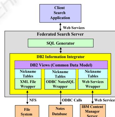
Figure 3: Implementation of a federated search server based on IBM DB2 Information Integrator and wrapper technologies.
