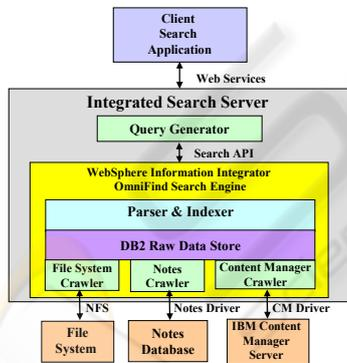
Figure 5: Implementation of an integrated search server based on IBM WebSphere Information Integrator OmniFind search engine.
