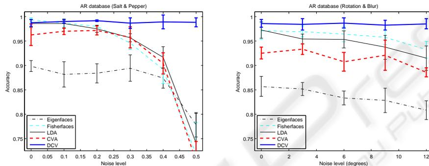
**Fig. 8.** Results obtained with the AR database with increasing levels of a) salt and pepper and b) rotation and II blur noise using all the classification methods considered.
