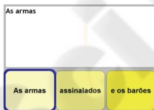
Figure 5: Virtual keyboard used to evaluate interaction with one continuous control signal to move mouse cursor in one-axis and one binary control signal to make key selection.
