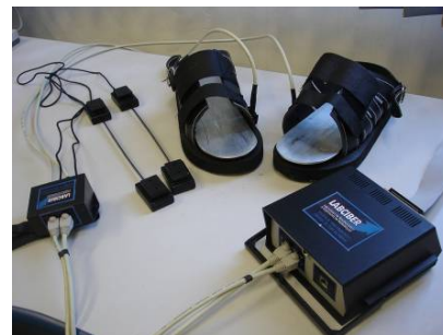
Figure 2: Transducers and patient's interface.
