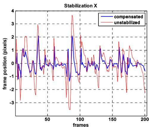
Figure 7: The red line presents each frame position before stabilization the blue line the stabilized one.
