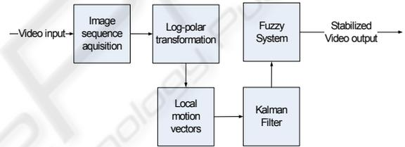
Figure 3: The block diagram of the proposed system.
