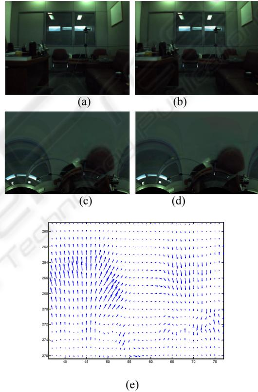
Figure 5: The optical flow field of two successive images (a) the first frame, (b) is the successive one, (c) the log-polar transformation of the first frame, (d) the log-polar transformation of the second one and (e) the optical flow, estimated on the log-polar plane.
