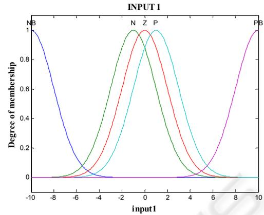
Figure 6: The membership functions of the fuzzy Kalman filter.
