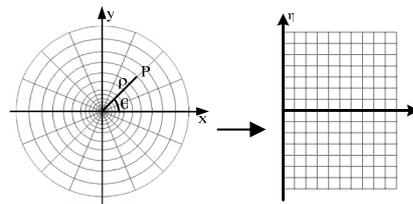
Figure 1: The log-polar transformation maps radial lines and concentric circles into lines parallel to the coordinate axes.
