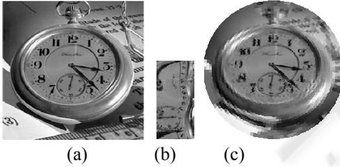
Figure 2: (a) Cartesian image; (b) log-polar image and (c) reconstructed Cartesian from log-polar image.
