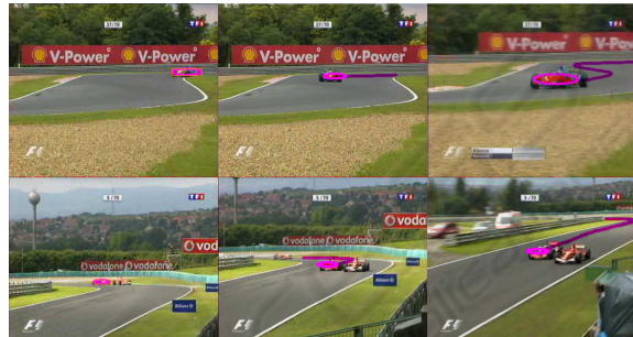
Figure 3: Images from video shots acquired by two different cameras at two different places on the circuit. The computed trajectories are overprinted on the images.
