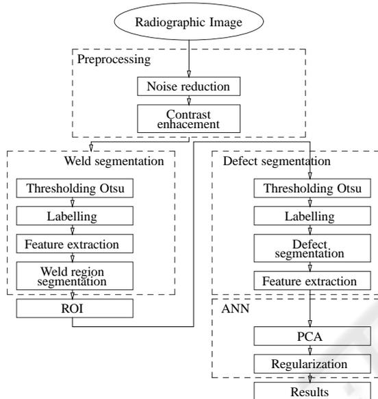
Figure 1: Procedure for the automatic welding defect detection system.
