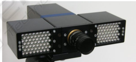
Figure 1: This figure shows the examined PMD Range Imaging Camera of model PMD [vision] 19k with the infrared LED matrices on both sides of the camera.
