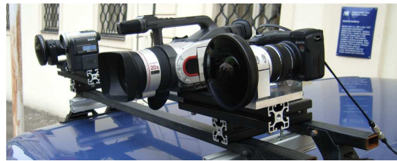
Figure 5: Kyocera Finecam M410R cameras with Nikon FC-E9 fish-eye lens convertors and two conventional perspective cameras mounted on a survey vehicle. Perspective cameras were not used in our experiments.
