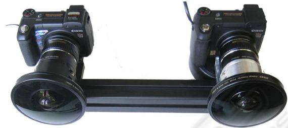
Figure 1: Omnidirectional stereo rig with Kyocera Finecam M410R cameras and Nikon FC-E9 fish-eye lens converters.
