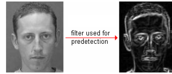
Figure 1: Predetection filter applied to a face image.
