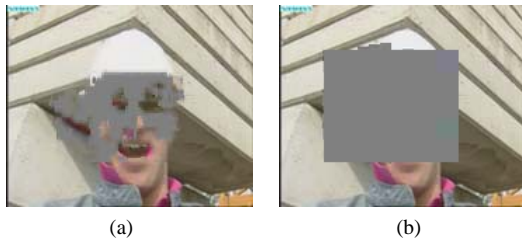
Figure 6: Decoded frame (Foreman QCIF) (a) without constrained inter-frame prediction (b) with limiting the search rectangle for ROI (ROI in grey).
