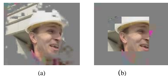
Figure 5: Decoded frame (Foreman QCIF) (a) without constrained inter frame prediction (b) with boundary padding of non-ROI (ROI in grey).
