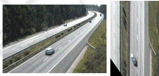
Figure 13: Example of a captured image (on the left) and the correspondent rectified image (on the right).
