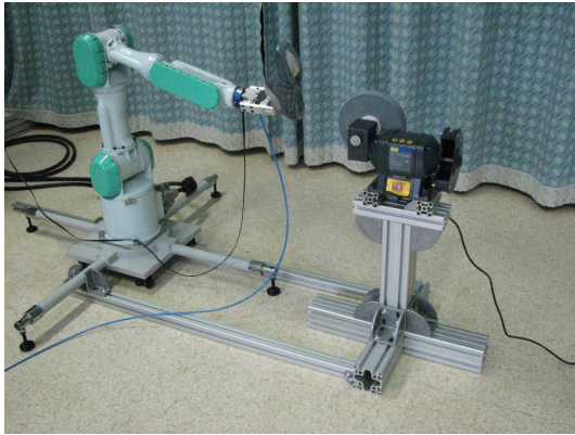
Figure 3: Experimental cell for shoe bottom roughing.
