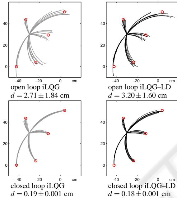
Figure 4: Illustration of the target reaching performances for the planar 2 DoF in the presence of strong control dependent noise, where  $d$  represents the average Euclidean distance to the five reference targets.
