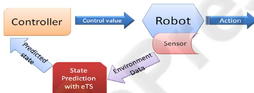
Fig. 5. System Structure of the predictive controller.
