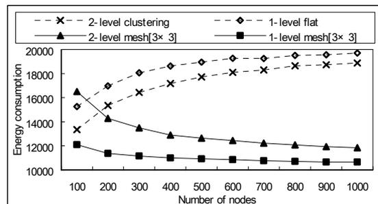
Figure 9: Energy consumption for different numbers of distributed nodes.
