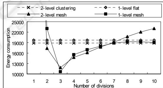
Figure 8: Energy consumption for different numbers of divisions.
