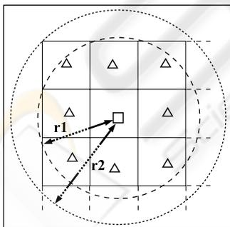
Figure 3: Two ranges in 2-level clustering and 1-level flat mesh approaches.
