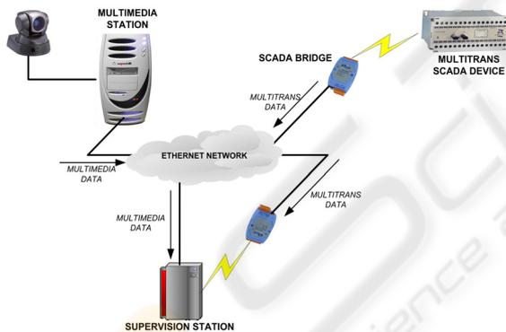
Figure 1: Ethernet SCADA bridge.
