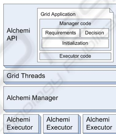
Figure 1: Alchemi Grid application architecture.
