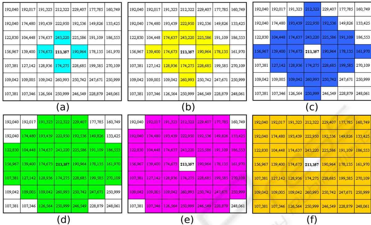
Figure 4: Six groups of pixels corresponding to the  $D_4$  metric distance classes on a  $7 \times 7$  texel on analysis: a)  $D_4 \leq 1$ , b)  $D_4 \leq 2$ , c)  $D_4 \leq 3$ , d)  $D_4 \leq 4$ , e)  $D_4 \leq 5$  and f)  $D_4 \leq 6$ .
