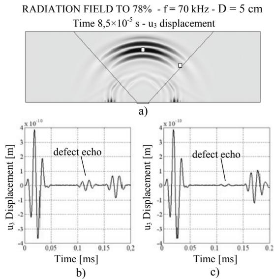
Figure 2: Comparison between  $u_3$  displacements: a) defects position; b) waveform for defect aligned with transducer axis; c) waveform for defect aligned with the radiation field border.
