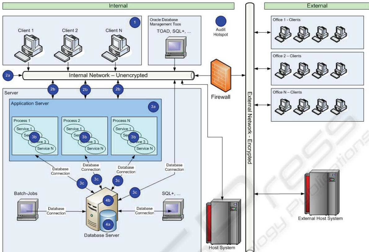
Figure 1: Audit-hotspot in a three-tier architecture.
