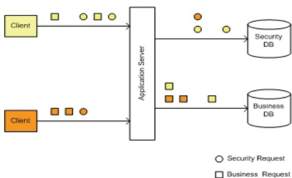
Figure 5: Connection pooling in a multi-tier environment.
