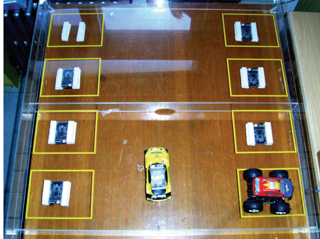
Fig. 7. The ubiquitous parking management system simulator with wireless sensors nodes and car model.
