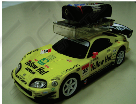
Fig. 4. The active RFID is placed on the top of the car model.
