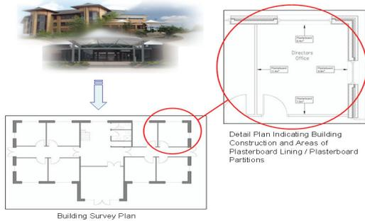
Figure 5: Surveying the Target Building and Indicating Plasterboard Materials.
