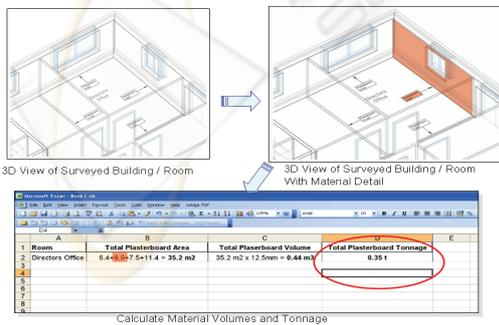
Figure 6: Predicting the Correct Volume and Tonnage of Plasterboard in Advance.
