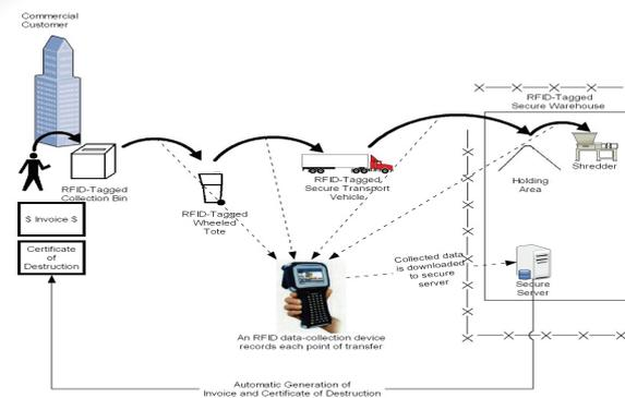
Figure 2: RFID-based Information to Automatically Generate Customer Invoices and Certificates of Destruction(NJE,2007).
