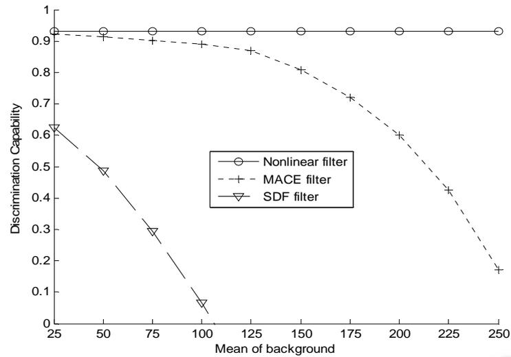
**Fig. 2.** Performance of filters in terms of DC as a function of the mean of background.
