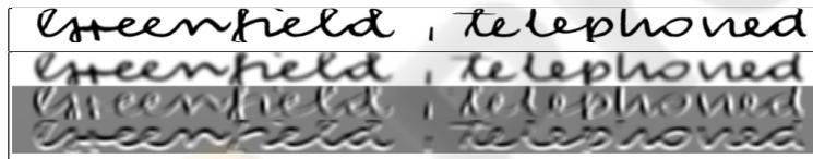
**Fig. 10.** An example of the graphical representation of the features extracted for the experiments (from up-to-down): preprocessed image, normalized gray level, horizontal gray level derivative, vertical gray level derivative.
