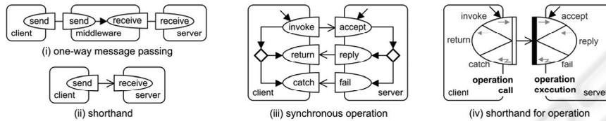
Fig. 6. Message passing and operation.
