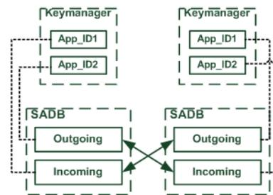
Figure 7: IPsec SADB and QKD Key Buffers.
