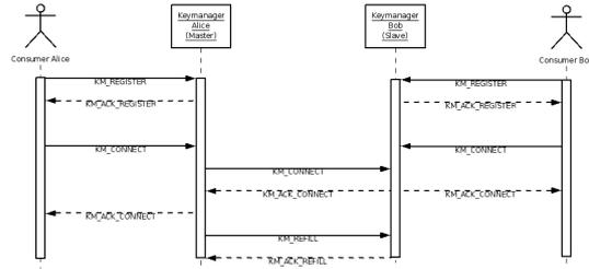
Figure 6: Message flow during connection establishment.
