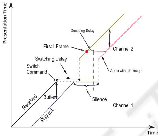
Figure 3: Switch resulting in an empty buffer due to late I-frame.
