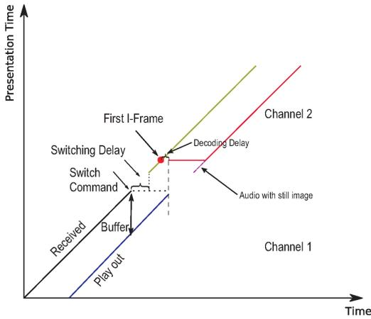
Figure 2: Switch without buffer underruns (optimal case).
