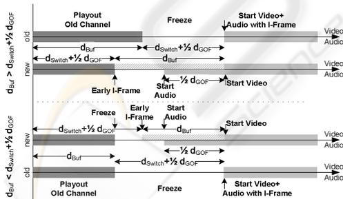
Figure 4: Multicast Switching - Simplified Playout Only.
