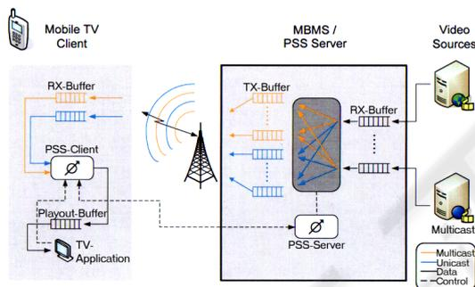
Figure 1: Proposed End-to-End Mobile TV Client/Server Architecture.
