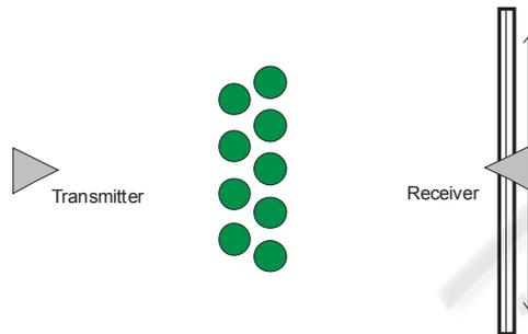
Figure 3: Zig-zag disposition (configuration 4).
