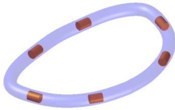
Figure 1: Active annuloplasty ring design. SMP with internal heating resistances. Biodevices 2008.
