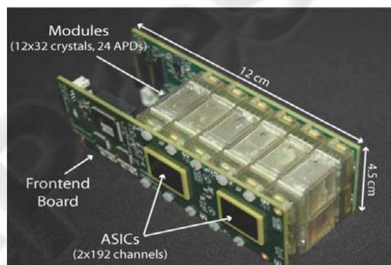
Figure 2: Supermodule structure assembling 12 modules, each with 32 LYSO:Ce crystals and two 32-pixel APD arrays in double readout. Each Frontend board has two ASICs with 192 input channels.
