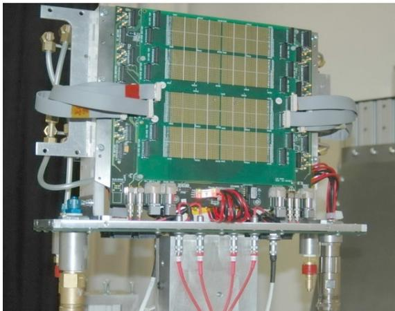
Figure 4: View of a detector head, with the hermetic patch panel on bottom, during the cabling phase.
