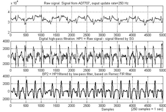
Figure 5: Record of the Q-SCG in normal man, age 45 years, 78 kg, after lowpass and highpass filtration. Raw signal is filtered by SG filter and Remez, finite impulse response (FIR) filter; 250 samples = 1 sec.
