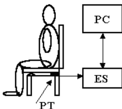
Figure 1: Principle of the noninvasive quantitative seismocardiography measuring: PT - piezoelectric transducer, ES - electronic system, PC - personal computer.
