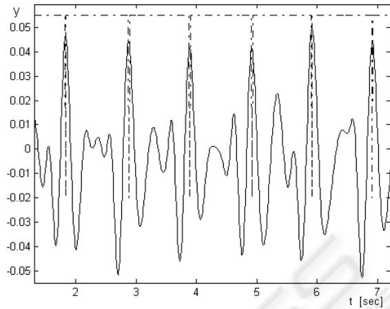
Figure 7: The heart rate variability can be also detected from Q-SCG signal.
