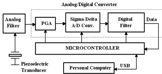
Figure 2: The simplified block diagram of the electronic system for Q-SCG measuring. The main parts of the system are: Piezoelectric force transducer, Analog Filter, PGA - programmable gain amplifier, Sigma-Delta A/D converter, Digital Filter, microcontroller and Personal Computer connected to system by means of USB (Universal serial bus).
