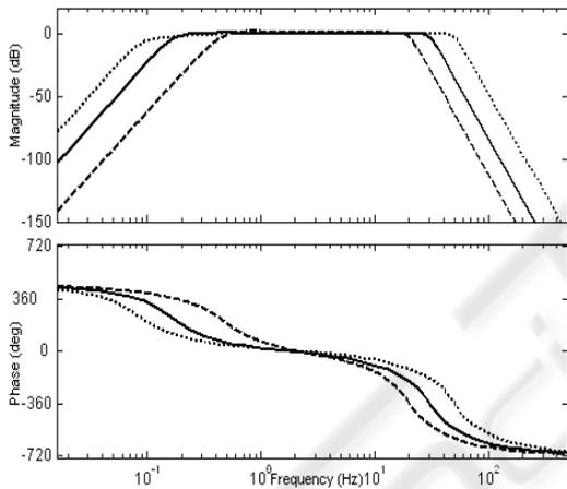
Figure 3: The frequency and phase responses of analog, electronically controlled filter.
