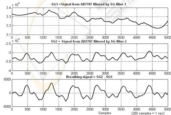
Figure 6: Breathing frequency derived from raw signal by means of two SG filters.
