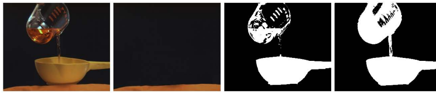
Figure 6: Comparison of background subtraction between gradient field based affine transform and kernel density estimation. Gradient field based background subtraction is more efficient in the area of illumination change or light's semi-transmission.
