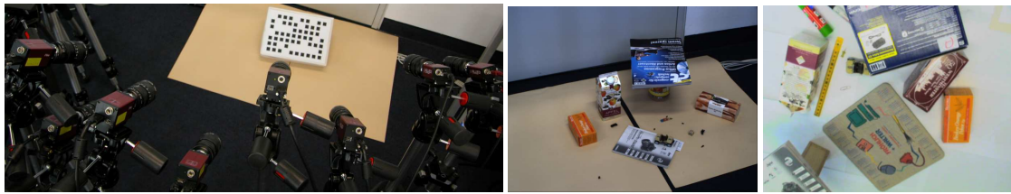
Figure 1: Experimental setups. Left: the multi camera system used in the first experiment observing the pattern for the Zhang calibration, middle: the according scene (image from the sixth camera), right: the scene used in the robot arm experiment.
