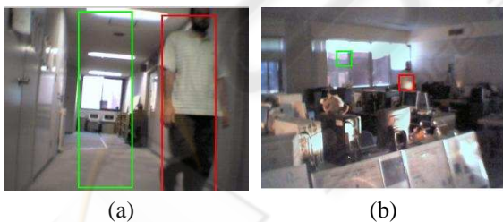
Figure 4: Kalman filter lost the object by wrong measurements.
