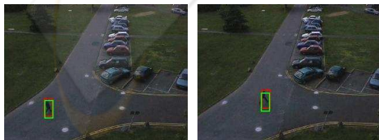
Figure 7: Image sequence four; Kalman tracker successfully tracked pedestrian in outdoor scenes guided by mean shift algorithm.
