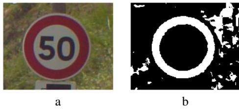
Figure 6: Image of a road sign (a) and detection by thresholding (b).
