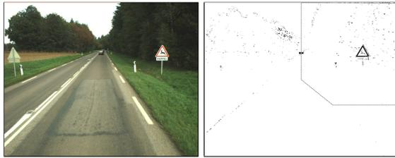
Figure 1: Road scene example (left); red/non-red pixel classification (right). The dotted polygon shows the search region for the selection of connected components. Pixels classified as red are shown in black.
