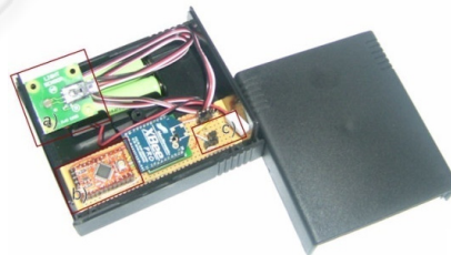
Fig. 3. Ambient device setup a) LDR sensor, b) microcontroller WEE, c) Temperature sensor.
