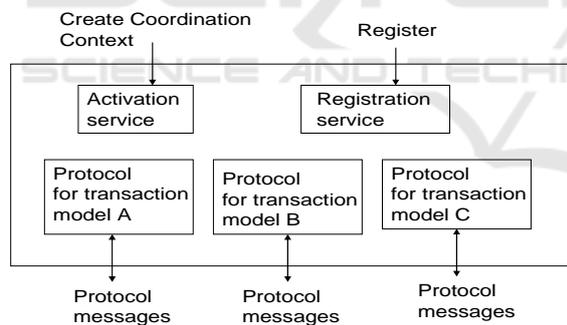
Figure 3: Coordinator for transaction models A, B and C.
