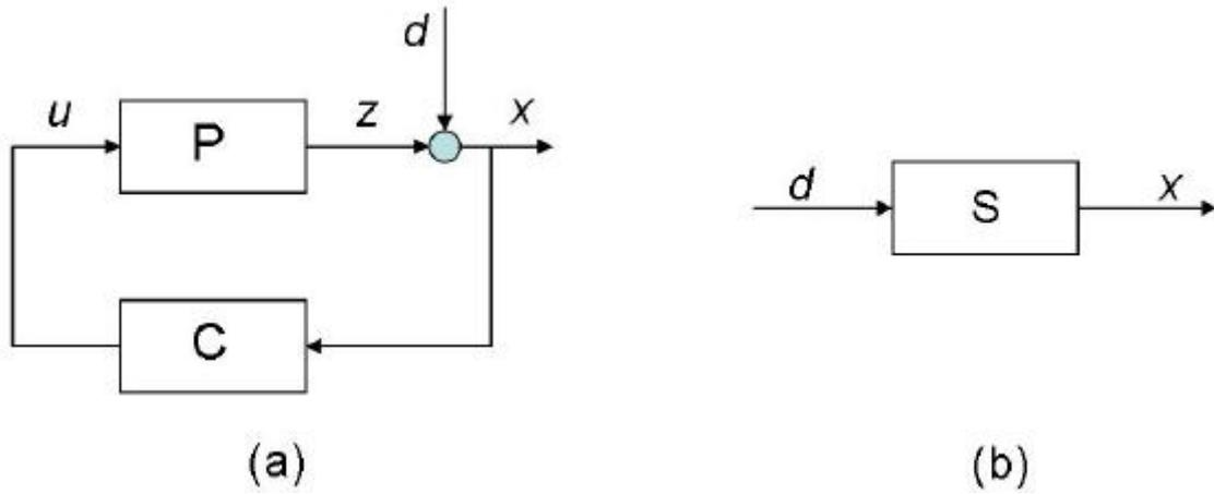
Figure 1: (a) Feedback loop and (b) Sensitivity function.
