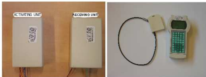
Fig. 4. Left picture: fixed reader solution with separated activator and receiver. Right picture: handheld reader with a closed electronic seal.
