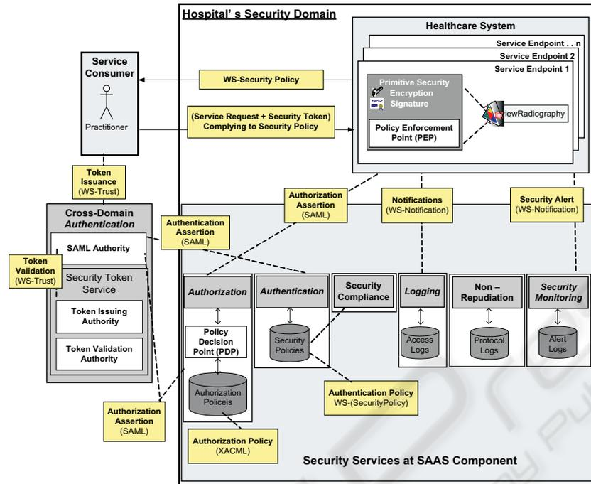
Fig. 3. The Reference Architecture.
