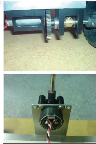
Figure 3: Geared DC motor (top) and Potentiometer (bottom).
