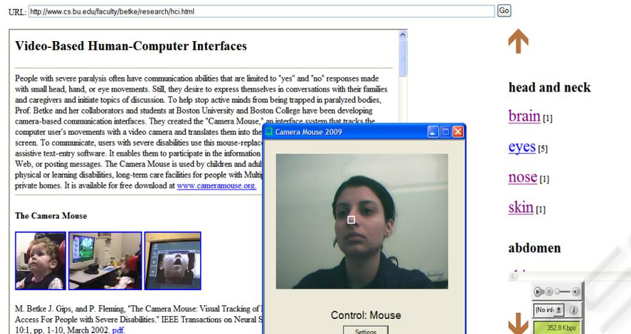
**Fig. 6.** Experimental Setup and testing phase of RefLink using CameraMouse. The small square shown in the CameraMouse interface indicates the selected feature to track, here the tip of the nose.
