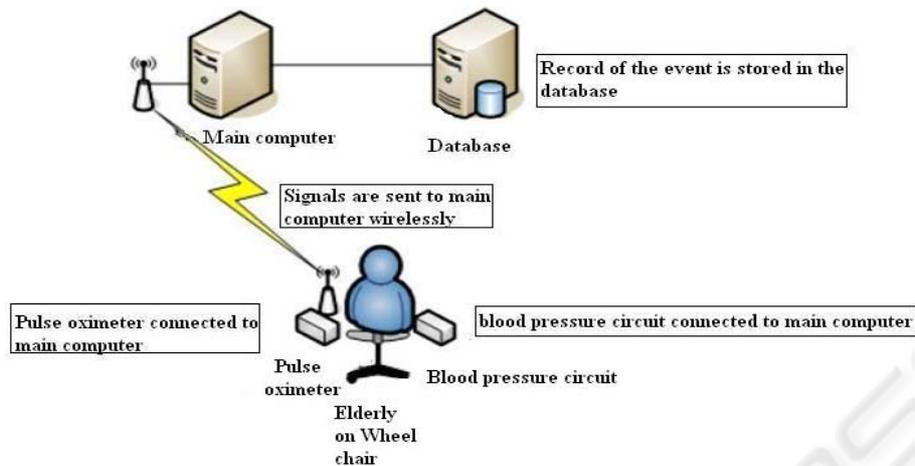
Fig. 2. Overall layout of the vital sign sensors.
