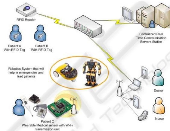
Fig. 4. The full layout of the mobile RFID based emergency system inside the hospital.
