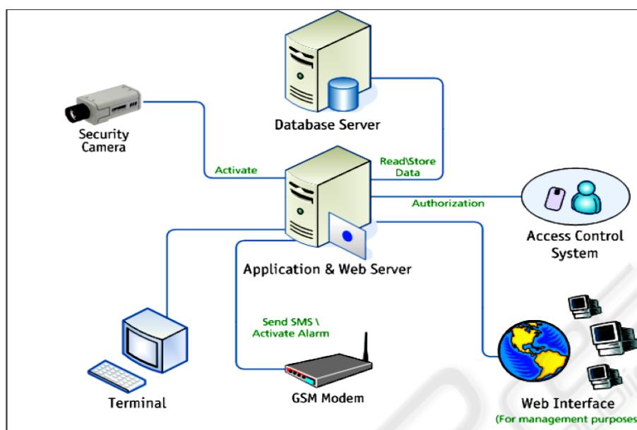
**Fig. 1.** An overall layout of the elderly monitoring system.
