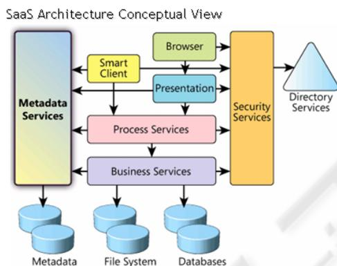
Figure 2: The architecture conceptual view of SaaS.
