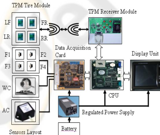
**Fig. 2.** Hardware structure of integrated prototype system.
