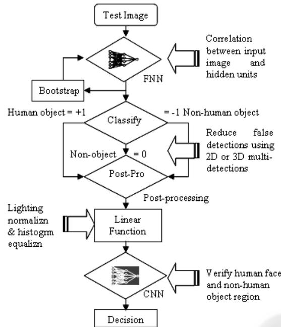
Fig. 1. Neural network algorithm for the occupancy detection.
