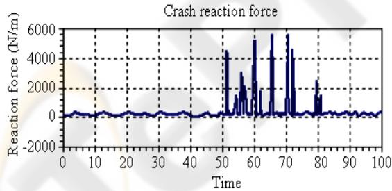
**Fig. 5.** Vehicle crash reaction forces.
