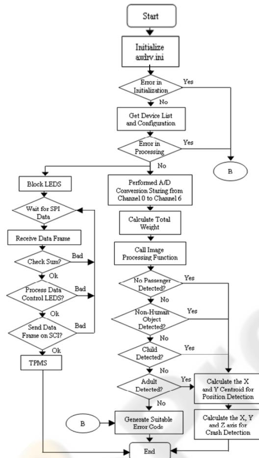
Fig. 3. Interface program flowchart of the integrated system.
