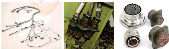
Figure 5: Connectors applied at an aircraft wire harness.
