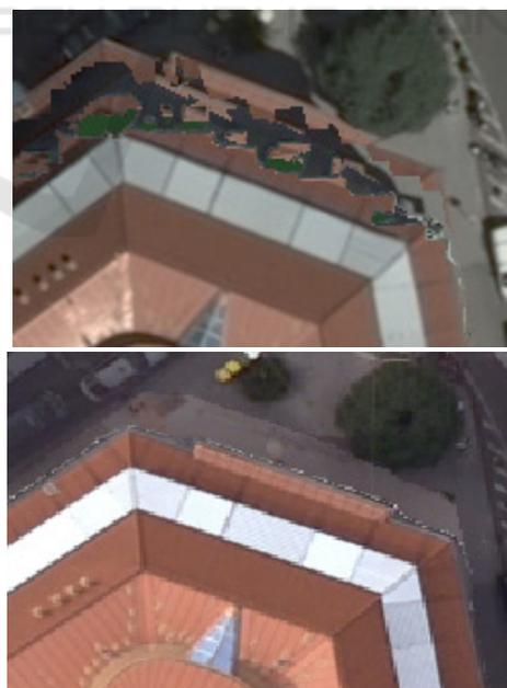
Figure 6: Segments of an ortho-photo. Above is the effect of a less well defined DSM, produced with an older DSM-algorithm. Below is the ortho-photo achieved with the DSM from the current state-of-the-art.
